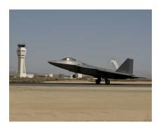
**Above:** An F-22 Raptor takes off from Edwards AFB to complete aerial refueling testing using an alternative jet engine fuel –a first for Air Force aircraft. The fuel is a 50/50 mix of jet fuel and natural gas-based fuel. (Lockheed Martin photo)
