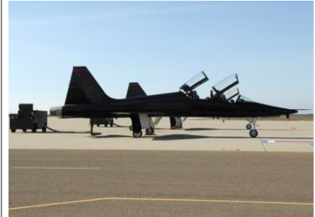
Above: The T-38 Talon is a twin-engine, high-altitude, supersonic jet trainer used in a variety of roles because of its design, economy of operations, ease of maintenance, high performance and exceptional safety record. (U.S. Air Force photo)
