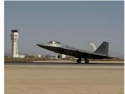
**Above:** An F-22 Raptor takes off from Edwards AFB to complete aerial refueling testing using an alternative jet engine fuel –a first for Air Force aircraft. The fuel is a 50/50 mix of jet fuel and natural gas-based fuel. (Lockheed Martin photo)
